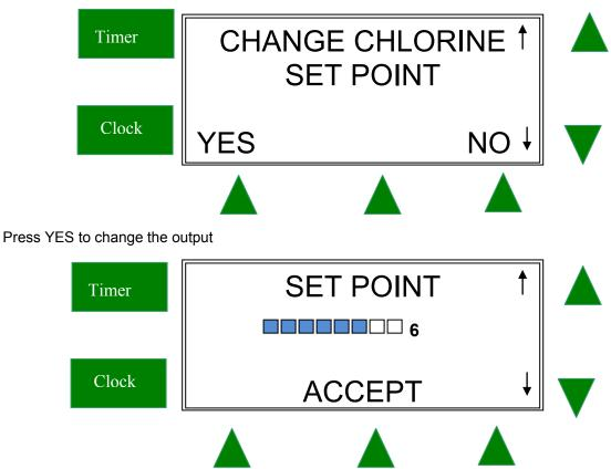
Press the SET button to change the chlorine output and the pH of your Pool
